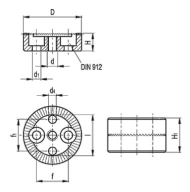
$$\begin{array}{lll} D & = 32 \\ d & = M6 \\ d1 & = 5.3 \\ d4 & H11 & = 5 \\ f & = 18 \\ f1 & = 18 \\ H & +/-0.9 & = 9.0 \\ H1 & = 18 \end{array}$$
